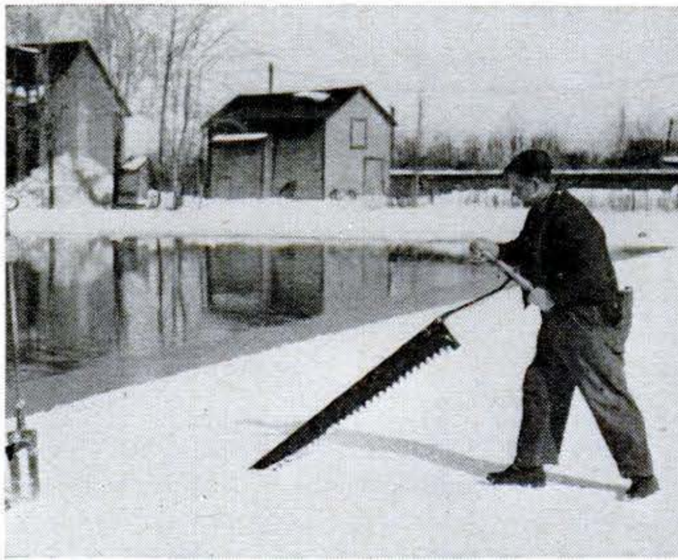
3. To provide room to work, first cakes are sawed by hand. End of the field is located upstream from storage house so that river current can help move ice down to conveyers.
